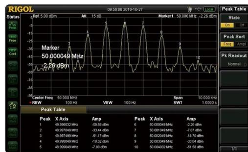
The advanced Harmonic distortion measurement function
