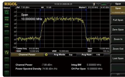
The advanced Occupied Bandwidth measurement function
