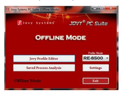
If standard profile is chosen, a new window will appear asking about type of board (leaded or lead-free) and profile parameters.
