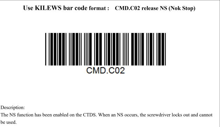
The operator can use Barcode Reader to scan the prepared command bar code to release it for easy operation.
