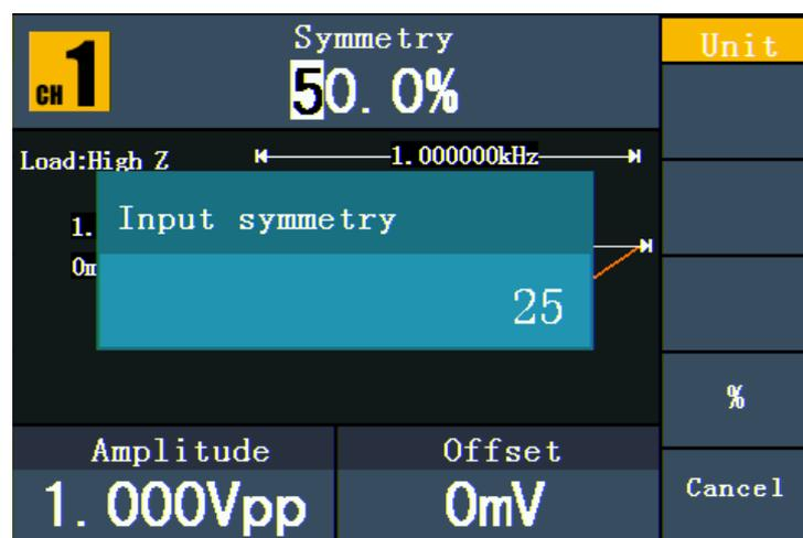
Figure 5-7: Set the symmetry of Ramp signal
