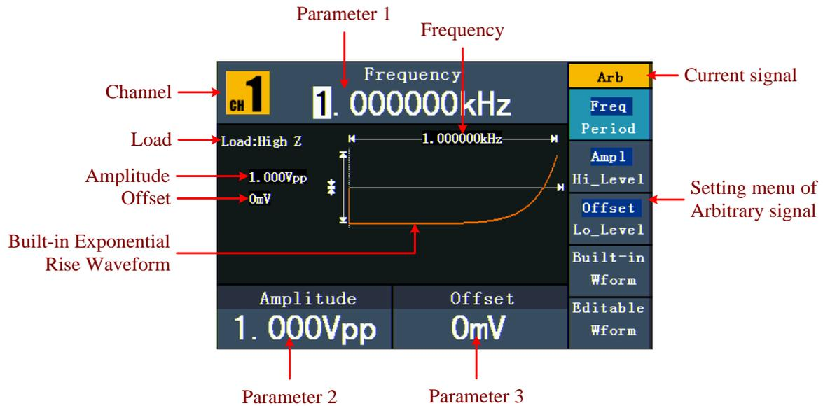
Figure 5-11: The User Interface of Arbitrary Signal
