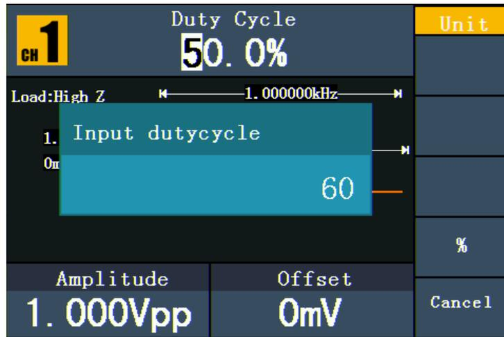
Figure 5-5: Set the Duty cycle of Square signal
