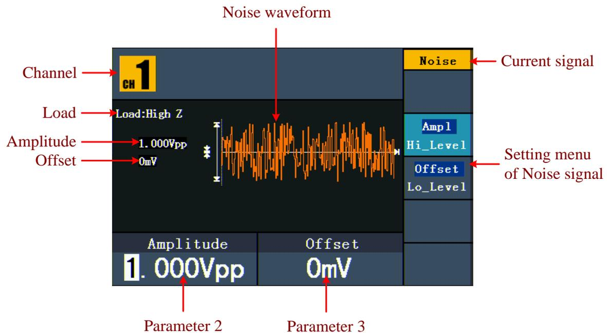
Figure 5-10: The User Interface of Noise Signal
