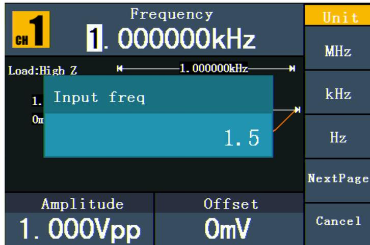
Figure 5-3: Set the frequency using number keys
