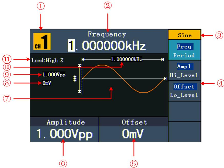
Figure 4-3 User interface (take Sine for instance)
