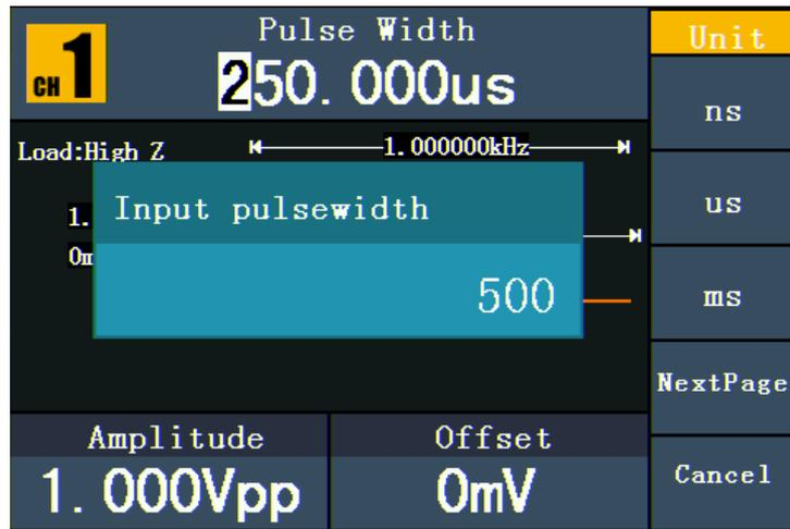
Figure 5-9: Set the Pulse Width of Pulse signal
