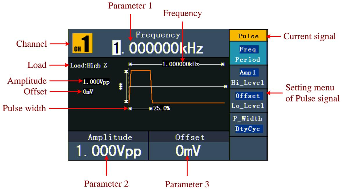
Figure 5-8: The User Interface of Pulse Signal
