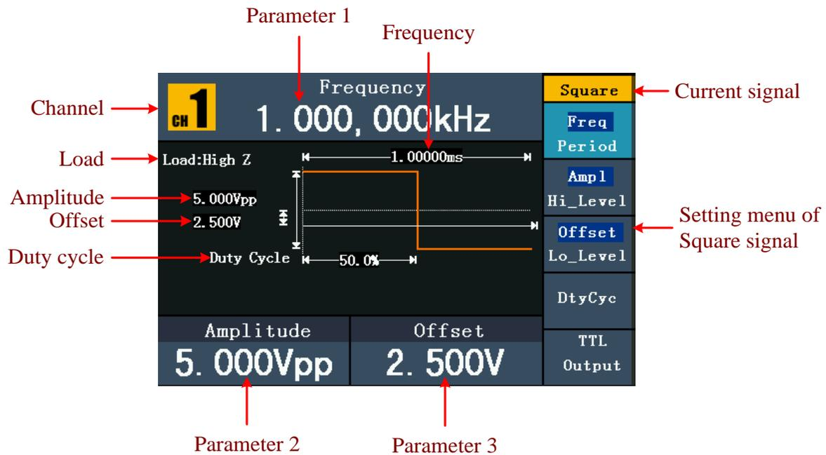
Figure 5-4: The User Interface of Square Signal
