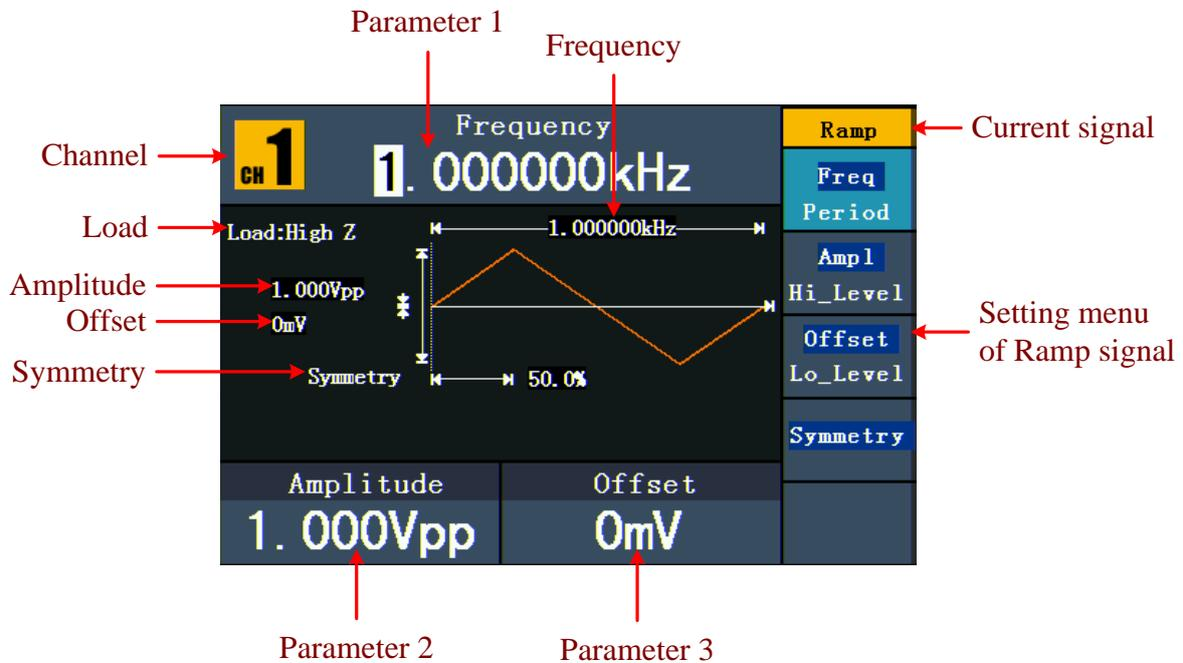
Figure 5-6: The User Interface of Ramp Signal
