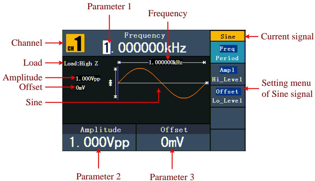
Figure 5-2: The User Interface of Sine Signal
