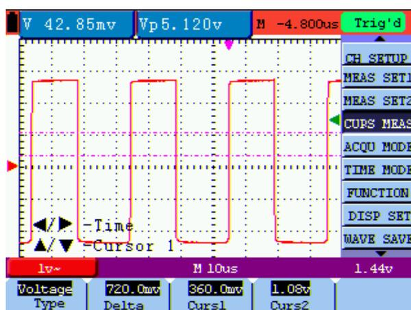
figure 45: Use the Cursor for a Voltage Measurement
