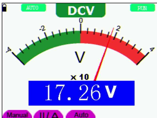
figure 22: DC Voltage Measurement
