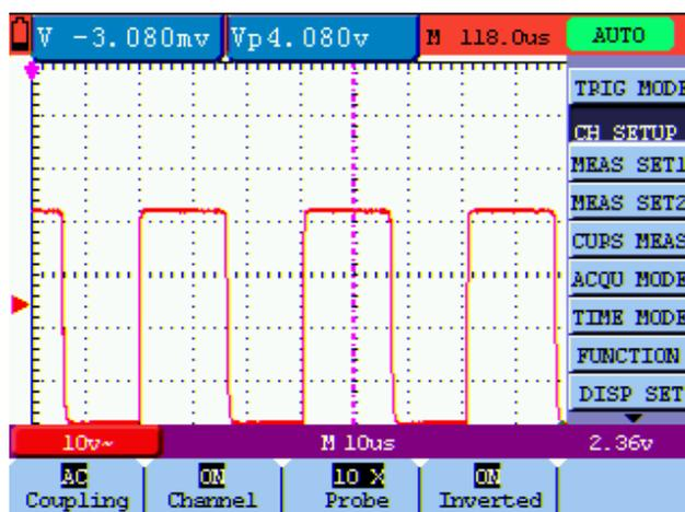
figure 16: Inverted On
