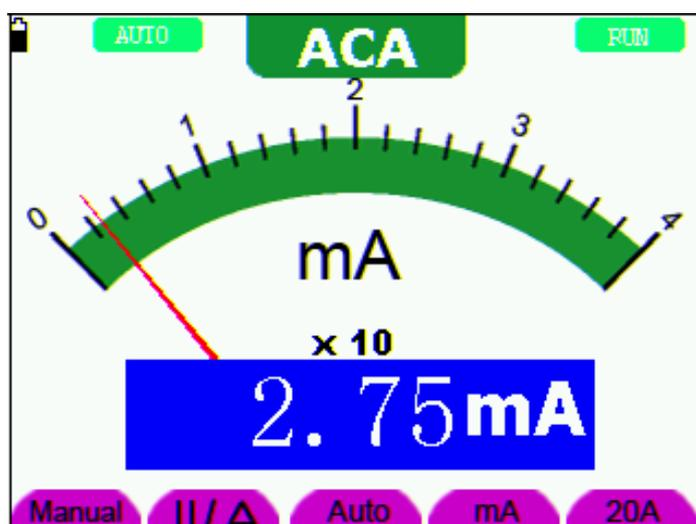
figure 26: AC Current Measurement for 400 mA
