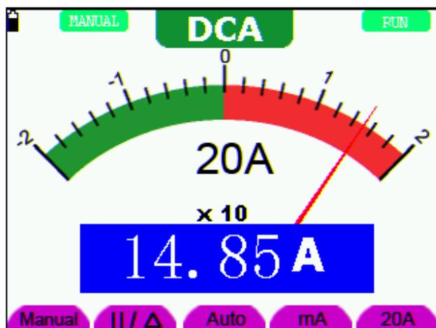
figure 25: DC Current Measurement for 20A
