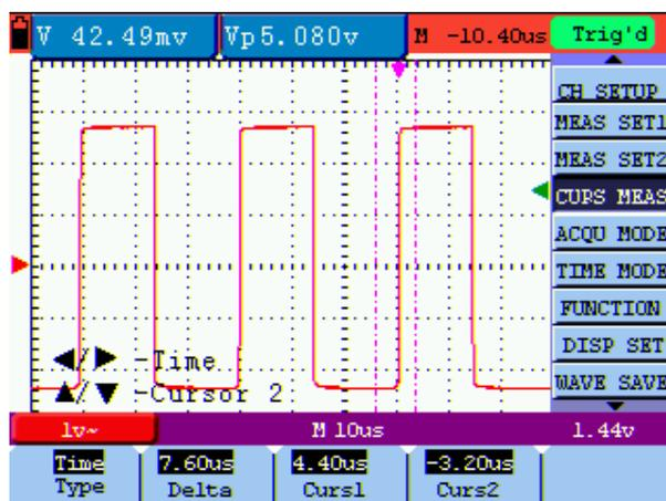
figure 46: Use the Cursor for a Time Measurement
