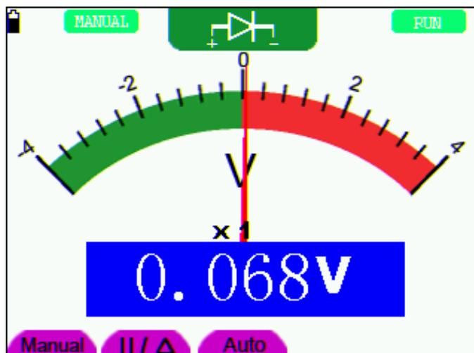
figure 19: Diode Measurement
