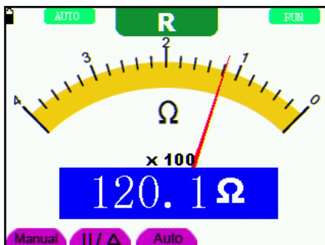
figure 18: Resistance Measurement
