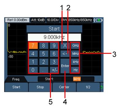
Figure 5-2 Numeric keypad interface
