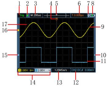
Figure 3-3:Oscilloscope Interface
