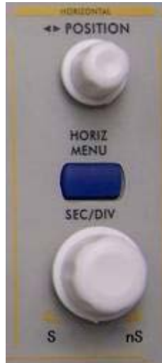
Fig. 4-10 Horizontal Control Zone
