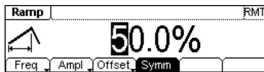
Figure 2-13 The Setting Interface of Ramp Signal
