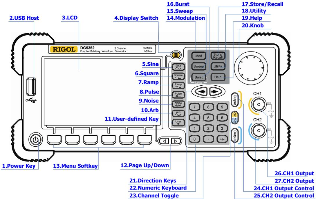
Figure 1-1 Dual-Channel Model Front Panel Overview
