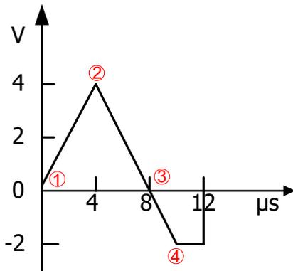
**Note:** As can be seen from the above figure, the waveform editor will always connect the voltage levels from the first point to the last point, and then maintain the level of the last point until the cycle period expires to create a continuous waveform.
