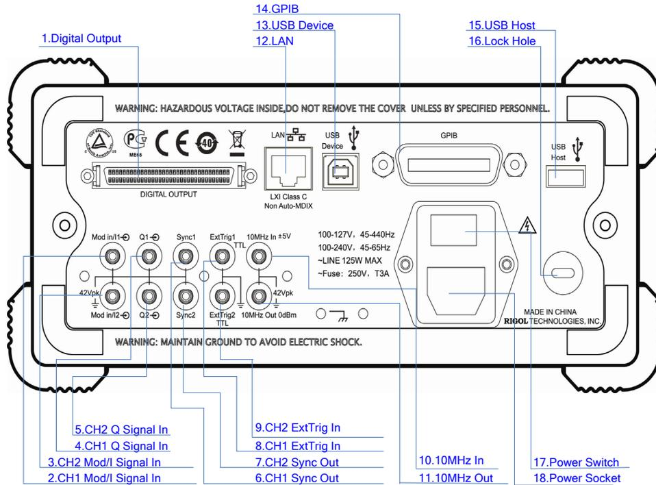
Figure 1-3 Dual-Channel Model Rear Panel Overview
