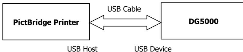
Set the Device Type to "Printer" (refer to **To Set USB Device Type**) and press **Pict Bridge** to enter the setting interface.
