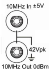
By setting clock source, synchronization can be realized between two instruments or more. "Align Phase" function is disabled when two instruments are synchronized as it only applies to align the phase relationship of the two channels in one generator. The phase relationship between two synchronous channels of different instruments can be changed by modifying the "Start Phase" of each channel after synchronization.
