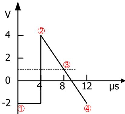
**Note:** As can be seen from the above figure, the waveform editor inserts values between the start point (point 2) and stop point (point 4) in the current interpolation method and then automatically generates point 1 and point 3 to create a continuous waveform.
