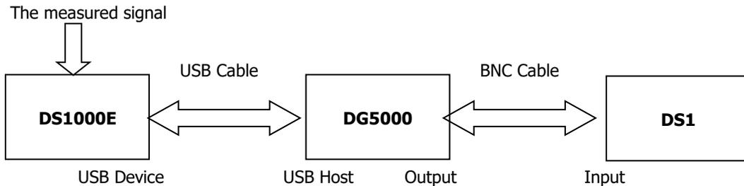
1. Make sure the measured signal is displayed stably on the screen of DS1000E.
