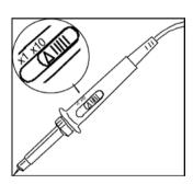
Figure 1- 11 Set attenuation on the probe
