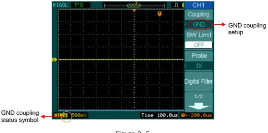
Figure 2- 5 GND coupling setting
