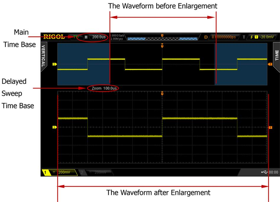
Figure 3-1 Delayed Sweep
