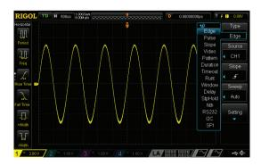
Built-in dual-channel 25 MHz source (DS1XX4Z-S Plus)
