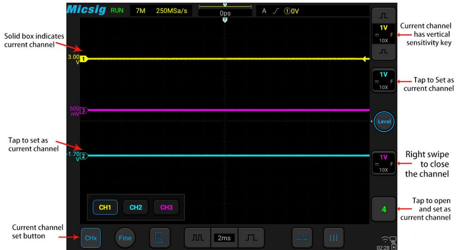
Figure 6-4 Channel Open, Close and Switching
