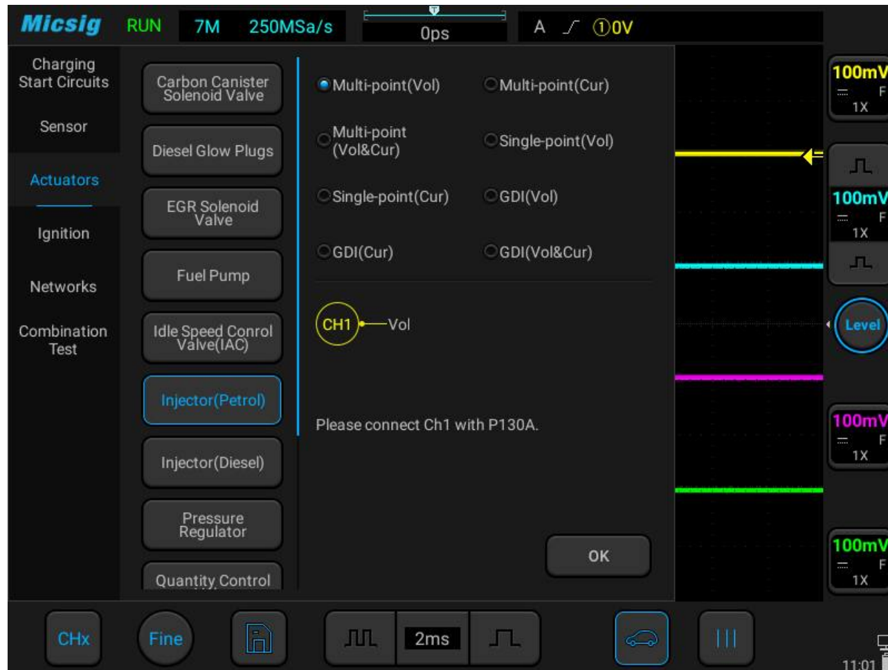
Figure 3-32 Injector (Petrol) Test
