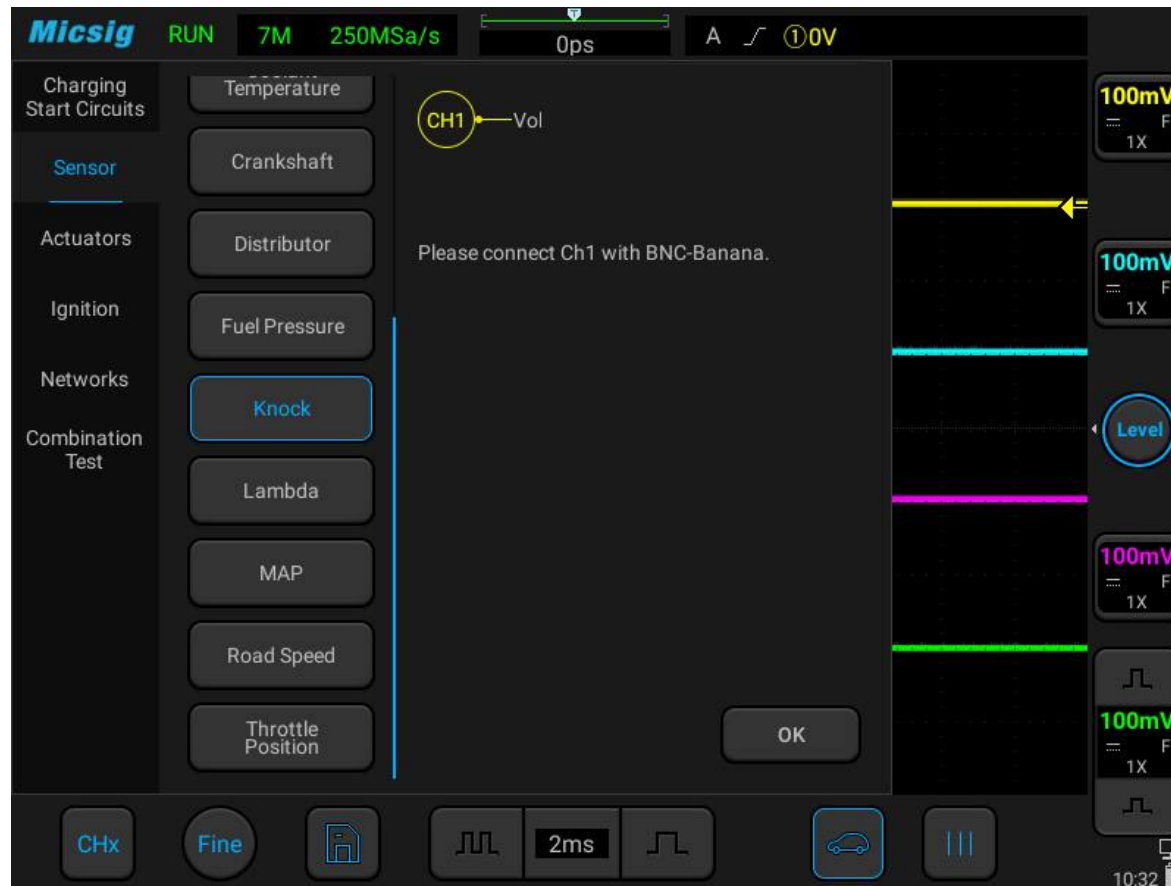
Figure 3-19 Knock Sensor test
