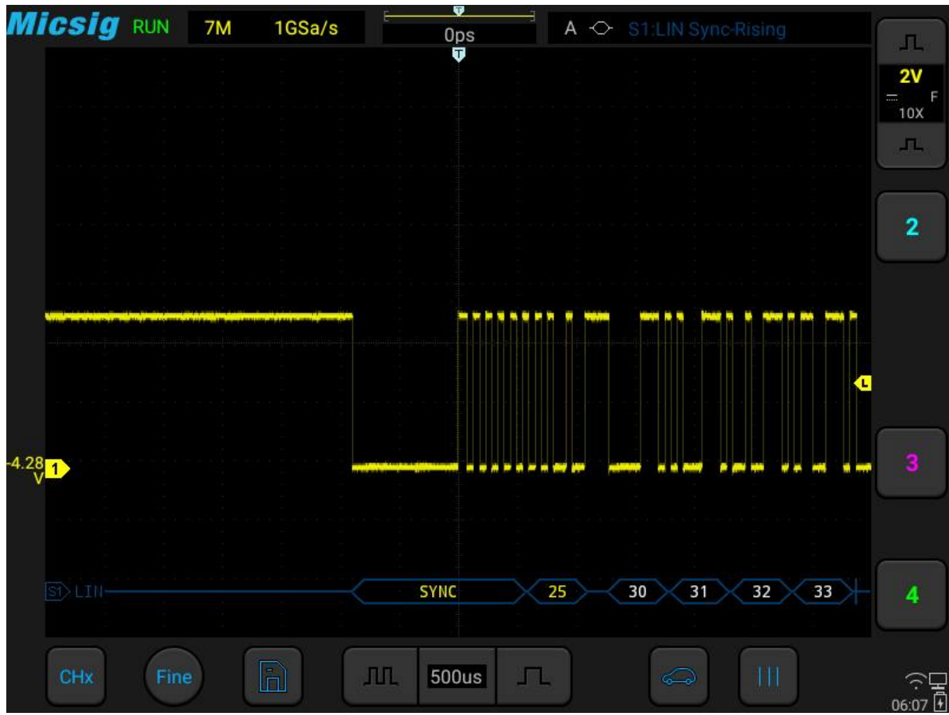
Figure 3-47 Audi A6 LIN bus measurement
