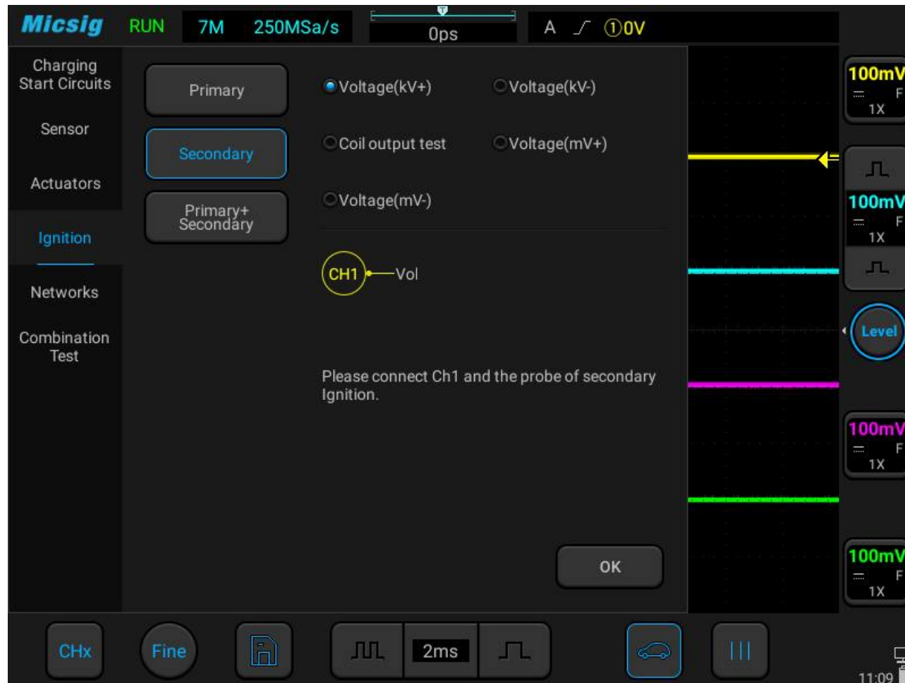
Figure 3-42 Secondary ignition test
