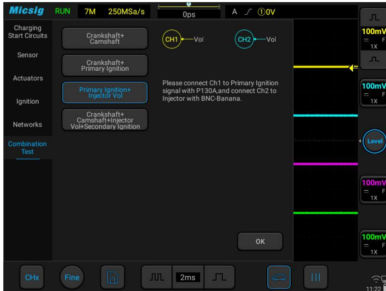
Figure 3-52 Primary ignition + Injector voltage
