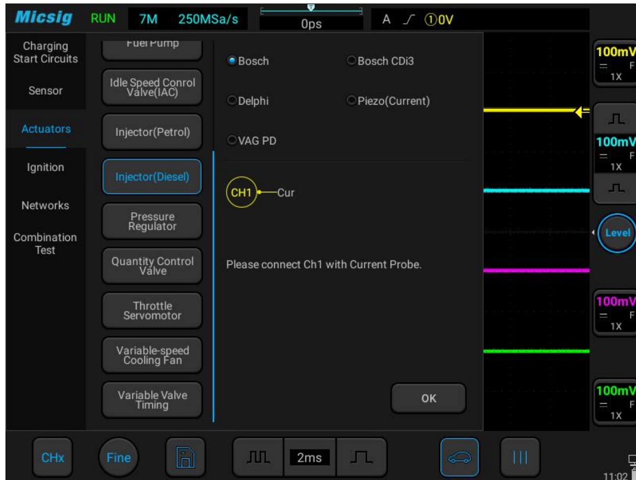
Figure 3-33 injector (diesel engine) test
