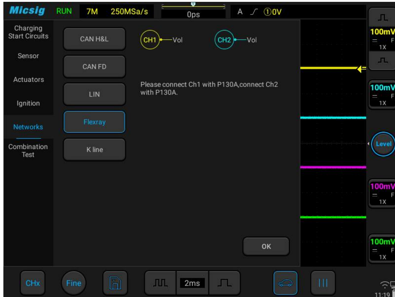
Figure 3-48: FlexRay bus test
