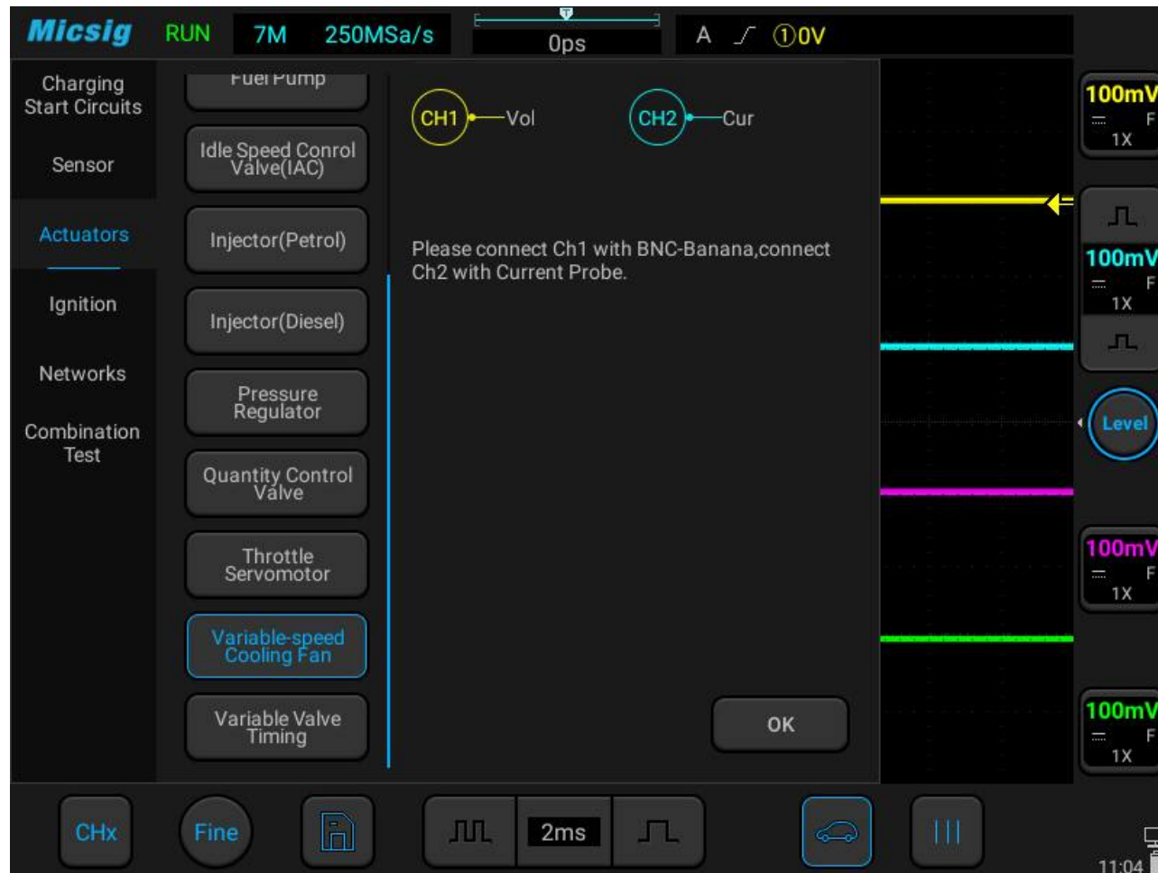
Figure 3-37 Variable-speed Cooling fan test
