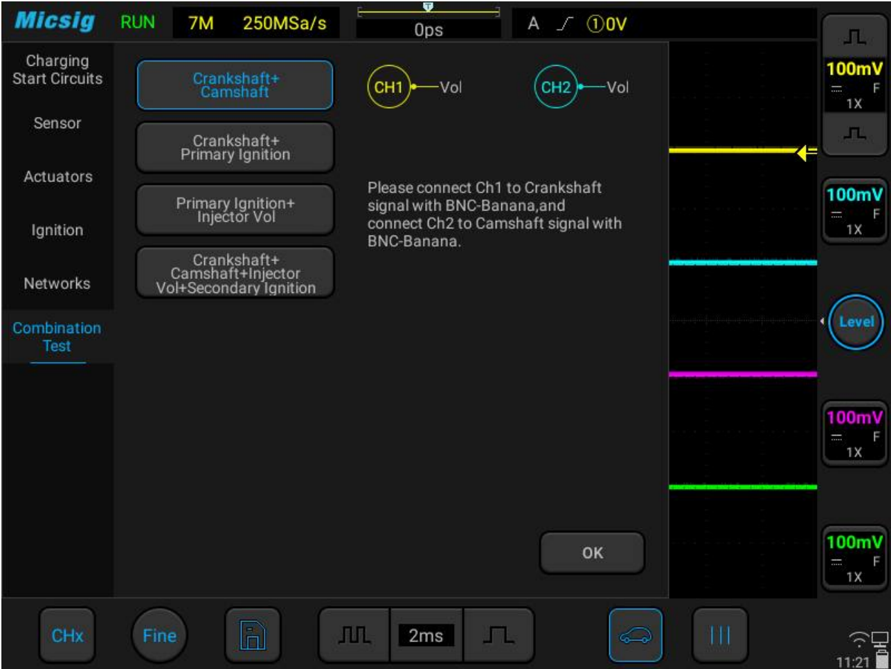
Figure 3-50 Crankshaft + Camshaft Combination Test
