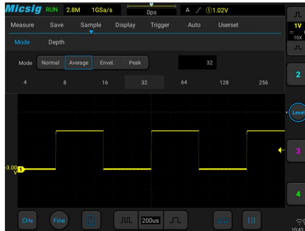
Figure 12-7 Waveform after choosing the average sampling mode, with average number 32
