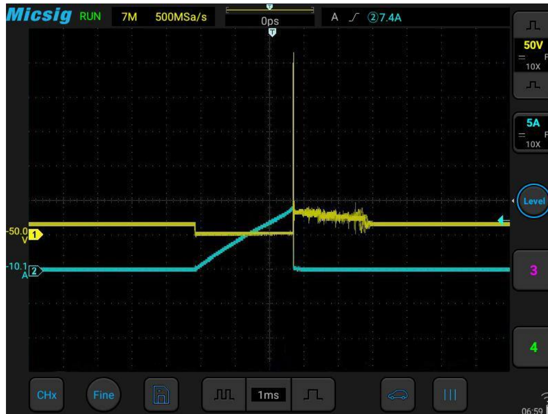
Figure 3-44 BMW 5 Series N20 Primary + Secondary ignition signal
