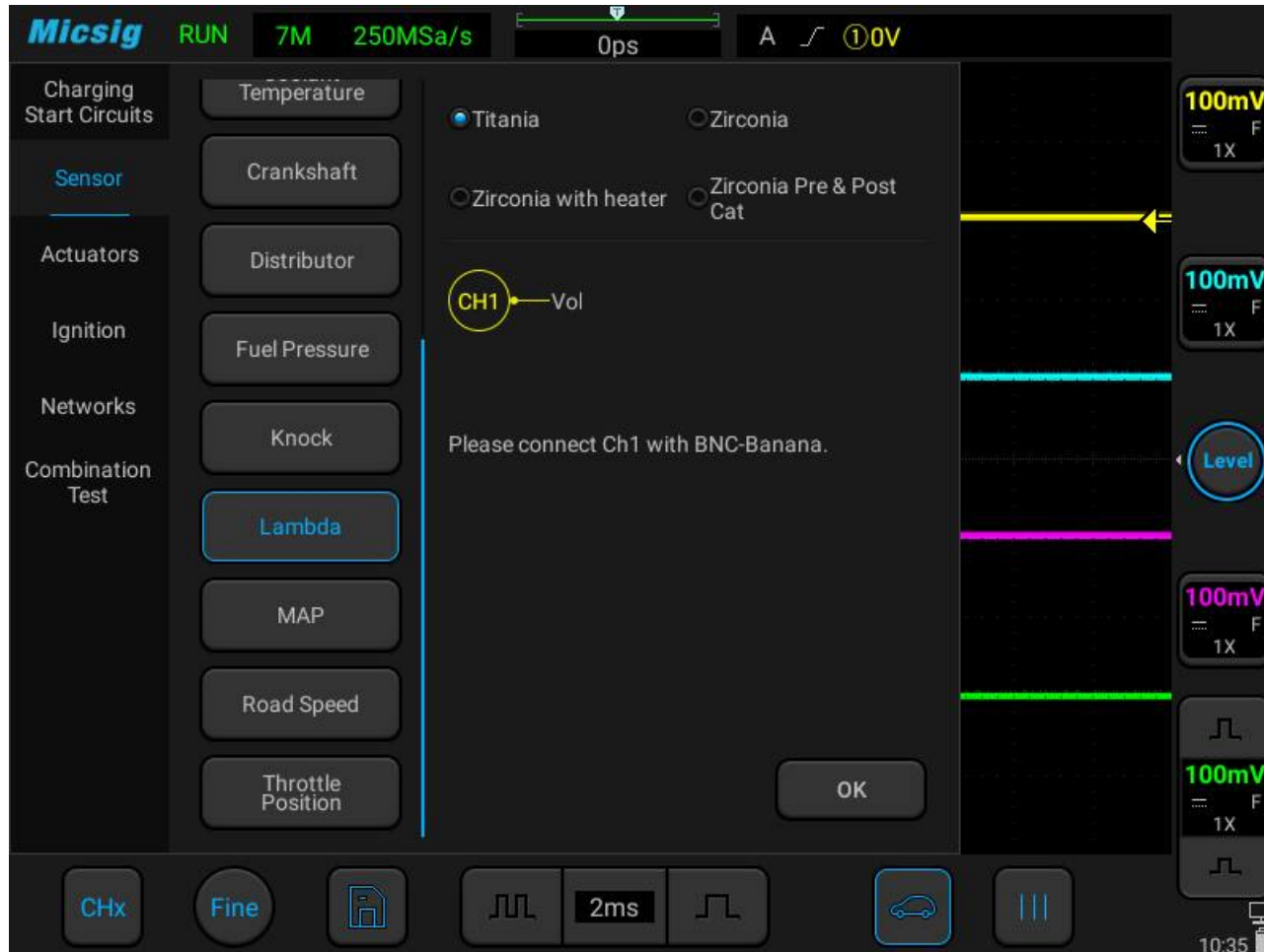
Figure 3-20 Lambda (oxygen sensor) test
