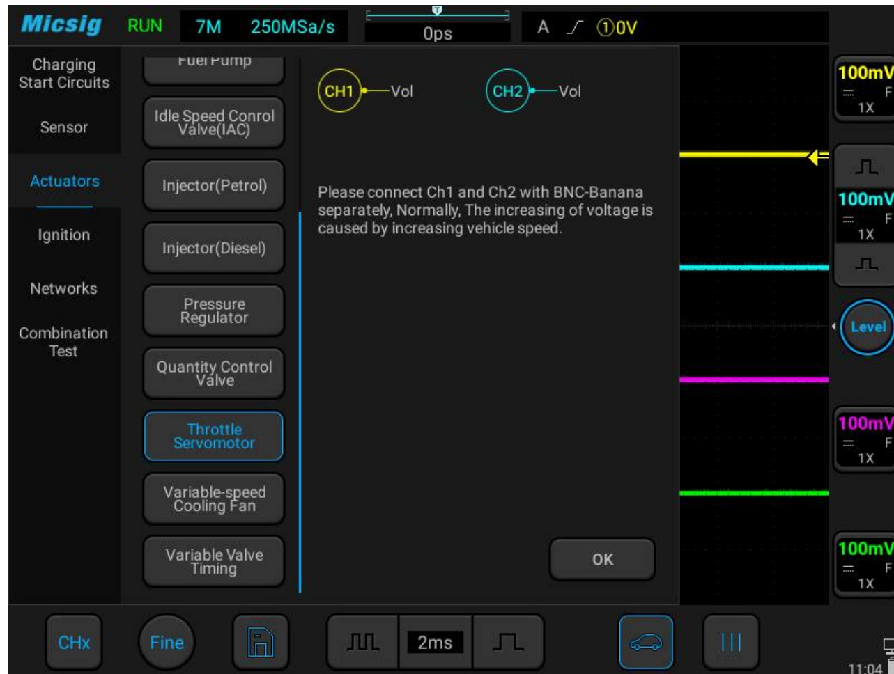
Figure 3-36 Throttle servo motor test
