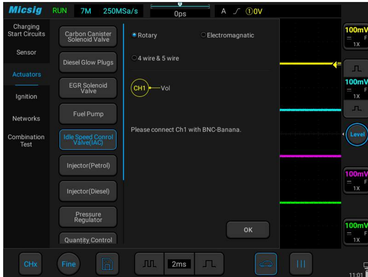
Figure 3-31 Idle speed control valve test
