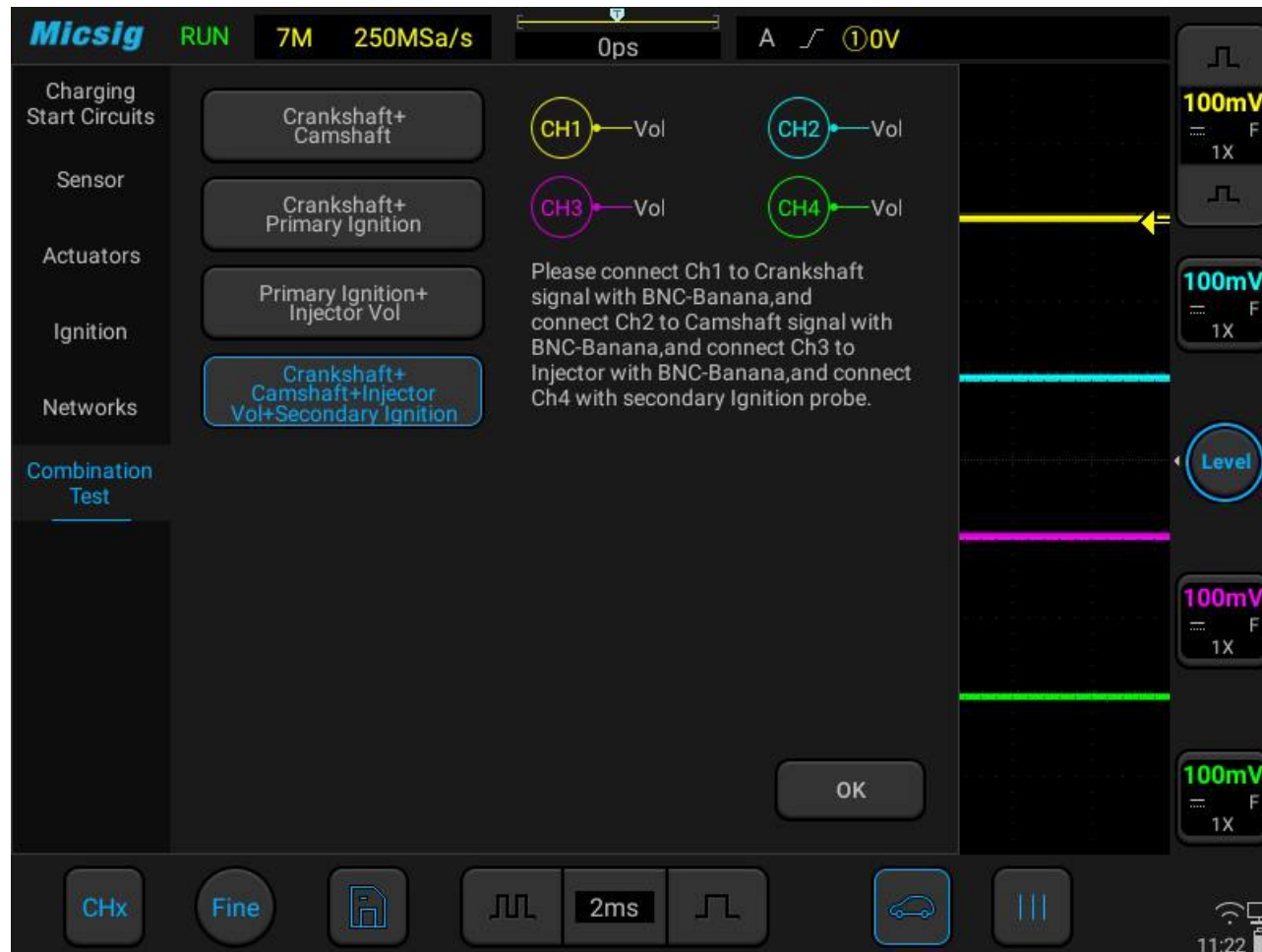
Figure 3-53 Combination test of Crankshaft + Camshaft + Injector + Secondary ignition
