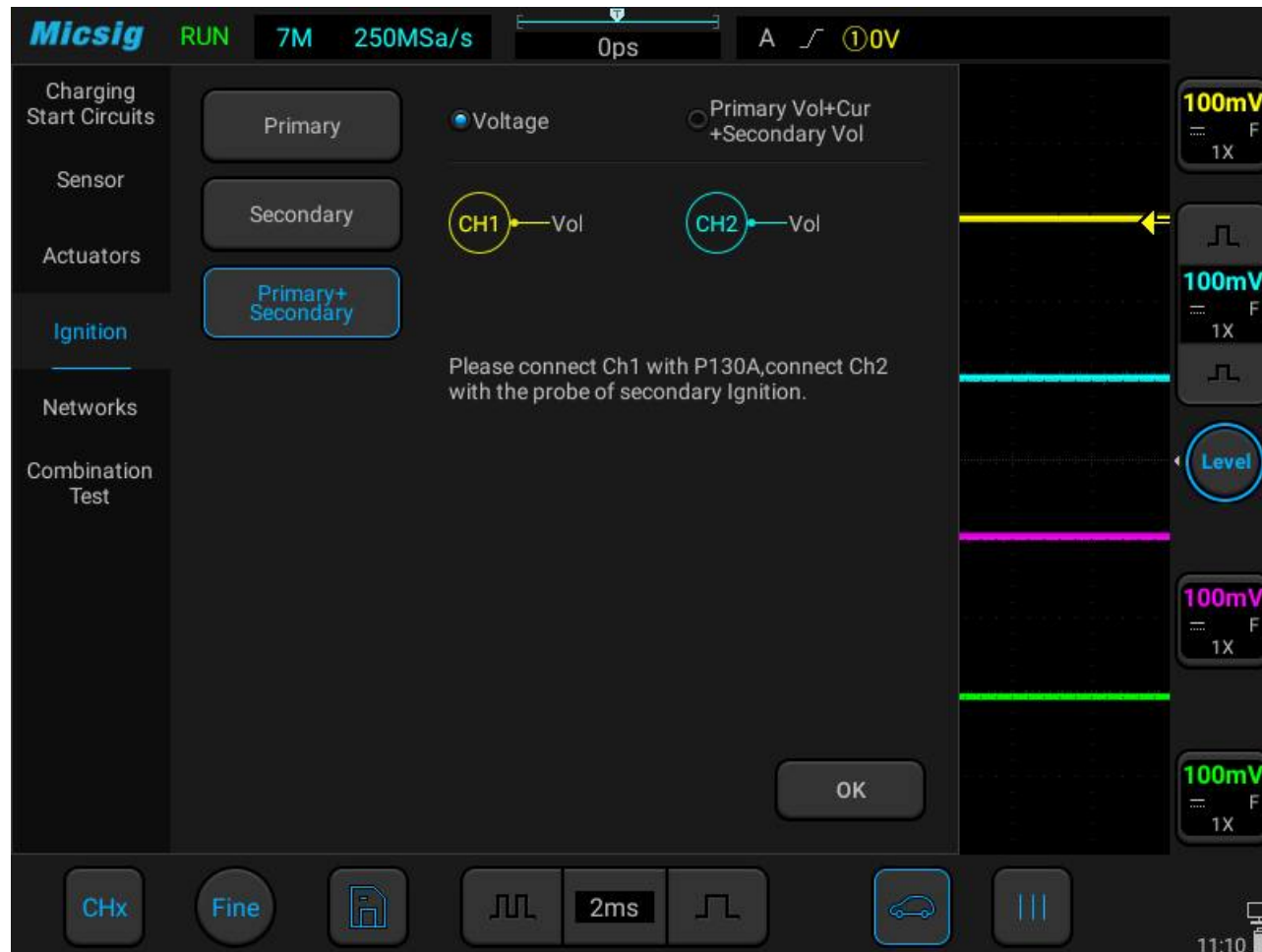
Figure 3-43: Primary + Secondary ignition test
