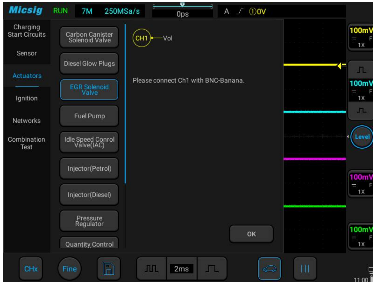
Figure 3-29 EGR solenoid valve test
