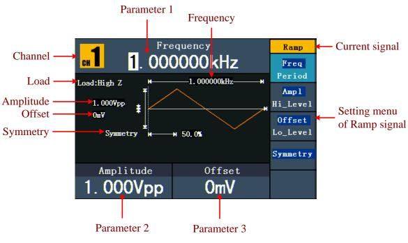
Figure 5-6: The User Interface of Ramp Signal
