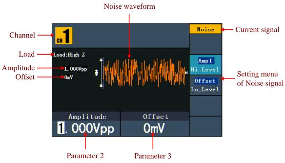
Figure 5-10: The User Interface of Noise Signal
