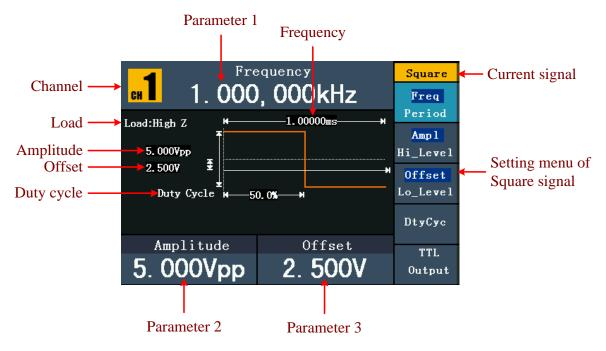
Figure 5-4: The User Interface of Square Signal
