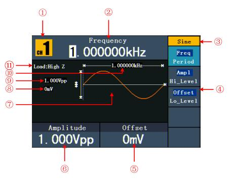
Figure 4-3 User interface (take Sine for instance)
