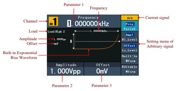
Figure 5-11: The User Interface of Arbitrary Signal
