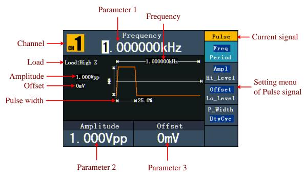
Figure 5-8: The User Interface of Pulse Signal
