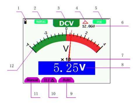
figure 17: Multimeter Operation Window
