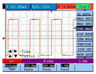
figure 45: Use the Cursor for a Voltage Measurement
