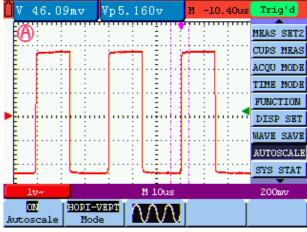
figure 47: Autoscale Horizontal- Vertical multi-period waveforms
