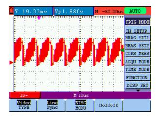
figure 36: Video Line Trigger
