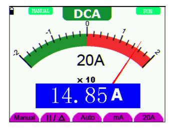
figure 25: DC Current Measurement for 20A
