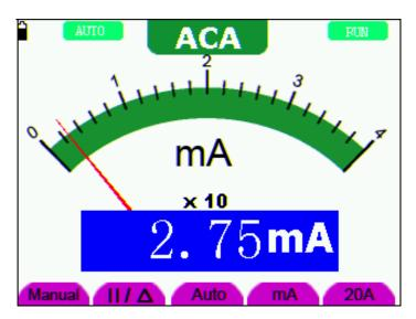
figure 26: AC Current Measurement for 400 mA
