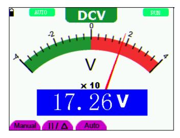
figure 22: DC Voltage Measurement
