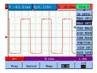
figure 44: Automatic Measurements
