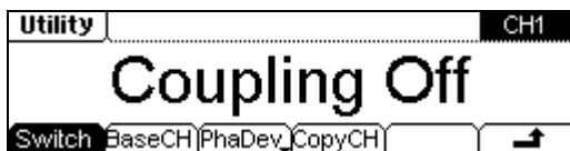
Figure 2-60 Channel Coupling Setting Interface
