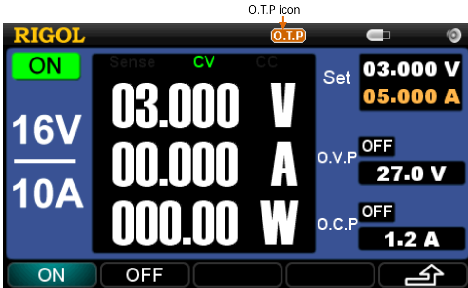
Figure 2-24 First Level Overtemperature protection setting
