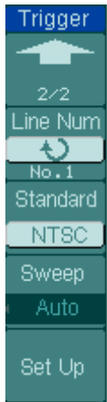
Figure 2-39 Table 2-21 The Video Trigger menu (Page 2/2, when Sync is set as the specified line)
