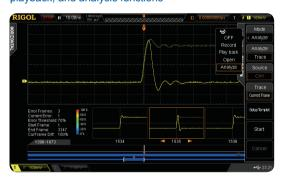
Serial bus trigger and decoding functions (supporting RS232/UART, I2C, SPI, CAN and LIN)
